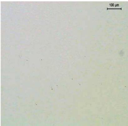
Fig. 4. Non-metallic inclusions stainless steel, longitudinal microsection magn. x100
